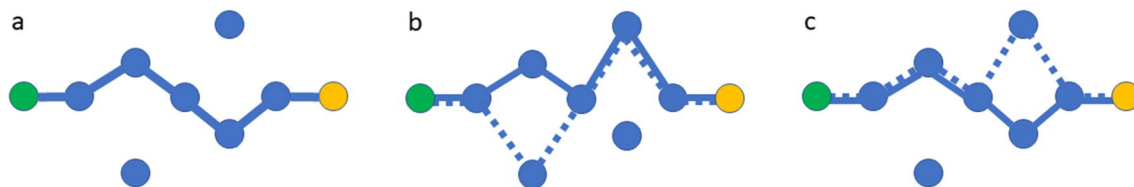
Fig. 1 a A set of nodes representing components of potential solutions to an optimization problem. Here, the edges connect the components of the globally optimal solution traversing from a start node (green) to an end node (yellow). b Agents probabilistically select paths that indicate candidate solutions. Paths associated with higher-quality solutions are reinforced (indicated by solid edges), making it
